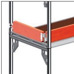
Fig. 35: Toe board insertion
