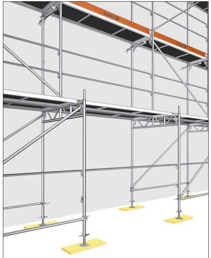
Fig. 105: Installation of gantry frames
