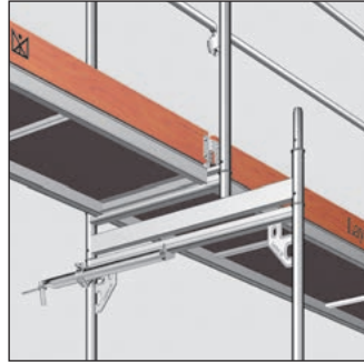
Fig. 107: Use of reducer
