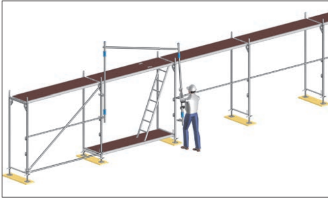
Fig. 25: Assembly of the advance guardrail in the access bay
