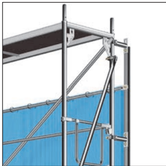
Fig. 130: Example for assembly of Keder tarpaulin system
