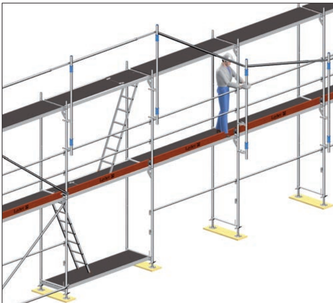
Fig. 26: Detail showing use of advance guardrail in the scaffolding level
